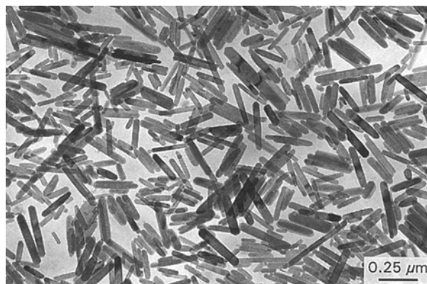
Figure 5 TEM photograph of rodlike \beta\text{-FeO(OH)} particles obtained by the hydrothermal ageing of fine \beta\text{-FeO(OH)} colloidal suspension ( [\text{Fe}^{3+}] = 0.3 \text{ mol dm}^{-3} ) at 120^\circ\text{C} for 6 h.
